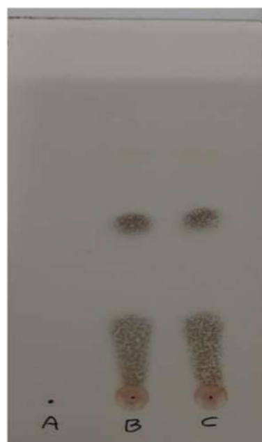
Fig. 2 High-performance thin-layer chromatography separation: A blank viscera; B viscera with carbaryl poisoning; C standard carbaryl
